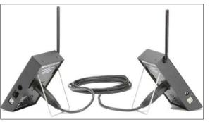
Interconnect with Cat-5 or 3-wire XLR cable or use DSan Part KES-882 to mix.
