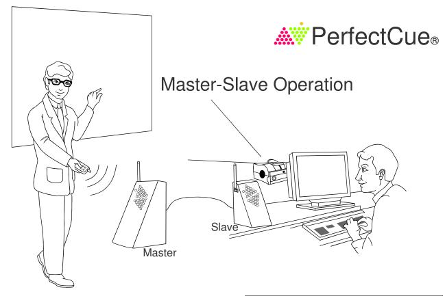
PerfectCue and PerfectCue Mini have RJ-45 and XLR jacks. Use Cat-5 (data) cable or XLR (microphone) cable to interconnect cue lights via these jacks. (Do not connect to audio equipment. Cables carry 12-V power.)
