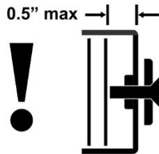
**Caution** when attaching VESA hardware. The total screw length from the outside of the case should be no more than 0.5". Use a washer or shorter screws. Correct side is M4 0.7mm thread. Consult DSan for alternate attachment screws.
