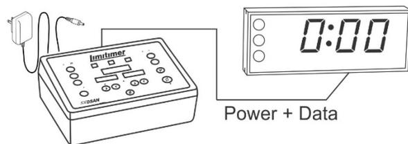
For cable runs greater than 100-feet, always provide local power to the signal light using the included 1-Amp power supply (center pin +).
