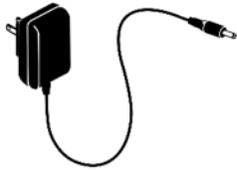
Signal light is supplied with a 12V 1Amp external power transformer that accepts 110-240 V mains fitted with the appropriate plug for your country. The timer and the signal light each draw approximately 300 mAmp. Therefore, it is possible to operate both the timer and up to 2 signal lights with one power supply. When the cable connecting the signal light to the timer is greater than 100-feet, the signal light should be locally powered.
